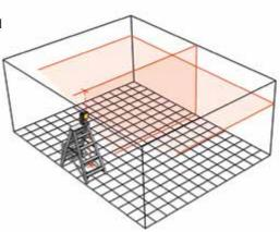
LAX 300: 1 horizontal laser line. 1 vertical laser line. Plumb up and down points.
