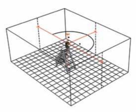
LA-5P: Plumb-up point, plumb-down point, level point, and square points.
