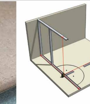
Fast layout and transfer of right angles. Up and down plumb points for the positioning of straight and curved studs.
