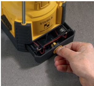
Battery drawer: Easy replacement directly on the tripod as well.
